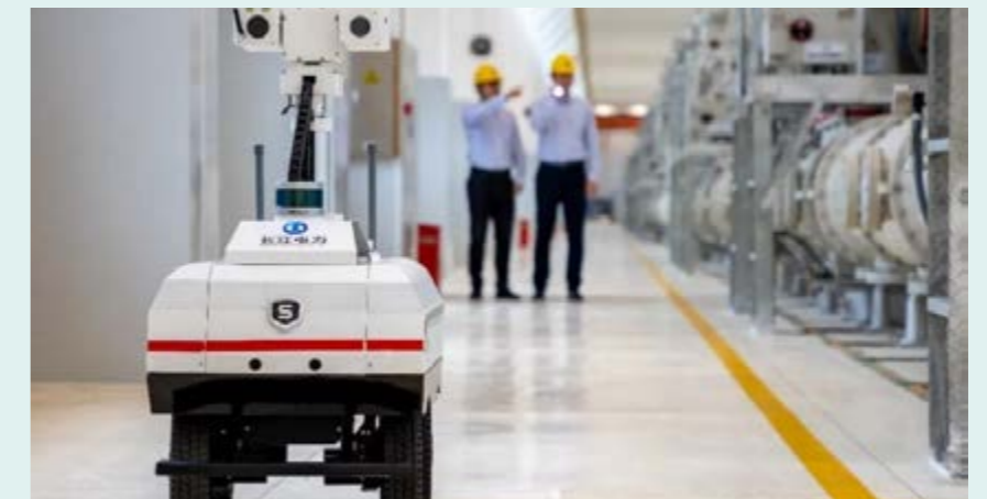
Patrol inspection robot "Xiaobai" is capable of automatic screening, precise early warning and timely elimination of hidden dangers
