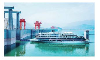
The ship has a 7,500 kWh power battery for ship use. Once it's fully charged, the ship can sail for 100 km. It is estimated that use of this ship can reduce carbon dioxide emissions by 1,600 tons per year.
